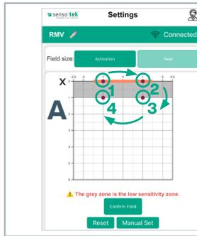
**Near area:** the gate will open in any case in this range. Set the points analogous to the activation range: **Point 1** on the x-axis (= zero line) to the **left** of the gate center, **point 2** on the x-axis (= zero line) to the **right** of the gate center, set **further points** in sequence (Fig. A), **not crosswise (left/right/left... Fig. B)! Save with "Confirm Field"** (Fig. C).
